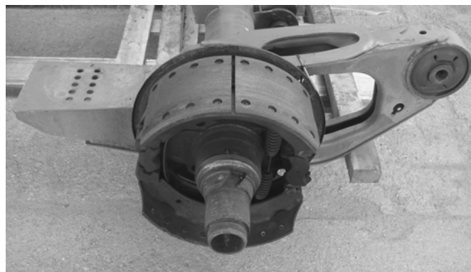
Fig. 2. Vehicle axle after 250 000 kilometres.
